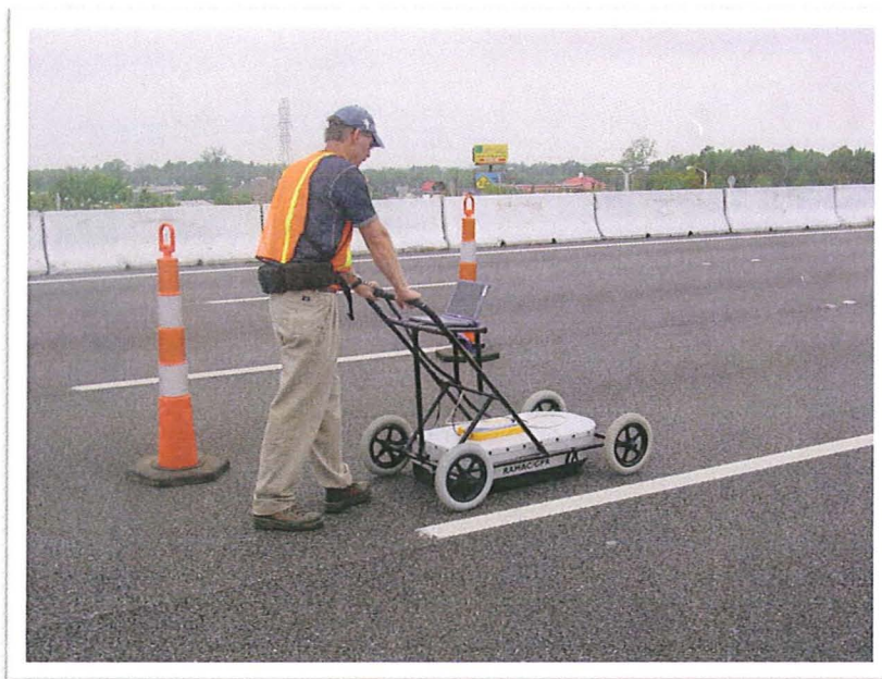
Underground utility survey using a ground penetrating radar (GPR) unit
